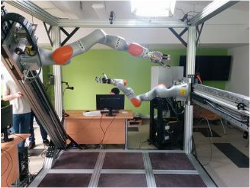
Fig. 3 Kube – the Kuka iiwa based universal research platform
