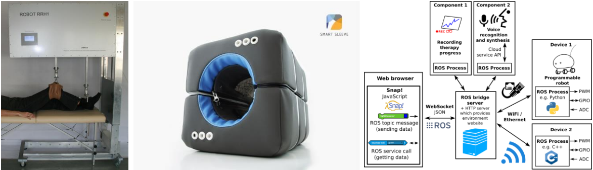
Fig. 1 Rehabilitation Fig. 2 Smart sleeve for sensory therapy and a structure of robot robot ROS based controller
