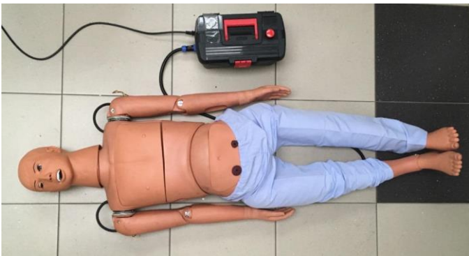
Fig. 4 Robotic phantom to imitate an epileptic seizure
